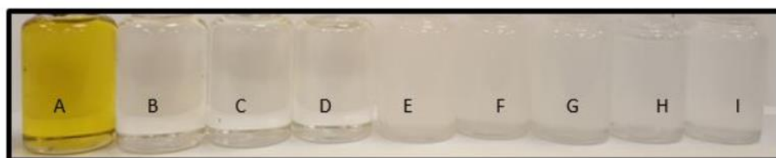
Figure 2. The change in the appearance of ozonated olive oil within hours (A: Initial, B: 3 h, C: 6 h, D: 9 h, E: 12 h, F: 15 h, G: 18 h, H: 21 h, I: 24 h).
