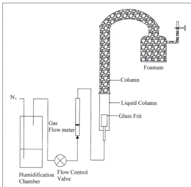
FIGURE 1. Schematic diagram of foam fractionation apparatus.
