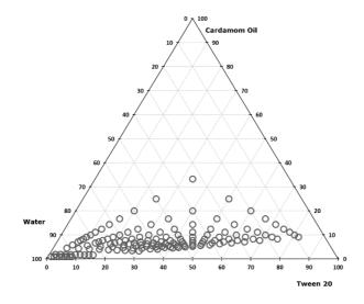
Figure 1. Pseudo ternary phase diagram demonstrating cardamom oil, tween 20, and water
