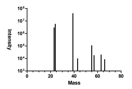
Figure 1. Representative ICP-MS spectrum obtained from sample E. The measured element lines; Na: 23 amu, Mg: 24 amu, K: 39 amu, Ca: 43 amu, Mn: 55 amu, Fe: 57 amu, Cu: 63 amu and Zn: 66 amu.
