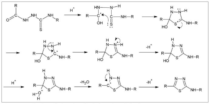
Scheme 2. Proposed mechanism for the synthesis of 2,5-disubstituted-1,3,4-thiadiazoles.
