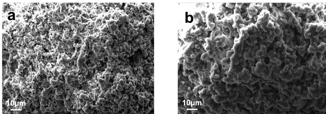
**Figure 2.** SEM images of nanoparticles : (a) pure PLGA/PEG nanoparticles (PNPs) and (b) CUR-loaded PLGA/PEG nanoparticles (CNPs)
