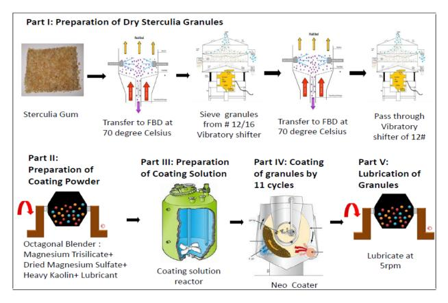
Figure 3. Manufacturing Process of Sterculia Gum Laxative Granules
